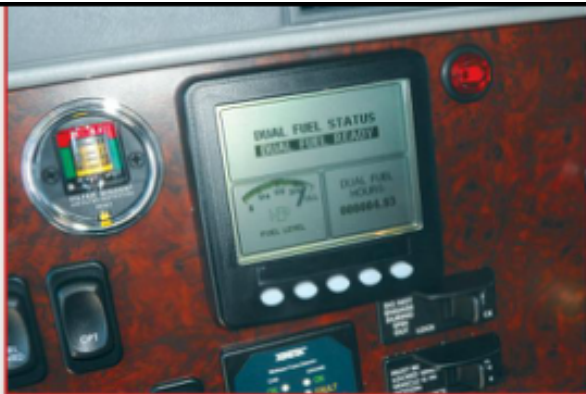
An LED readout offers various info on the natural gas fuel system's status. At idle, as now, no gas is being used, but the rate goes as high as 65% and averages about 50% while at highway speeds.
