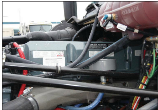
The Series 60 Detroit Diesel engine was refurbished and retrofitted with a bi-fuel natural gas kit from APG and Wheel Time before being dropped in a Freightliner Columbia glider.
