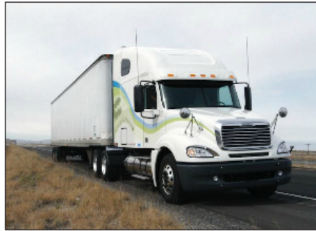
The 2014 Freightliner Columbia daycab was a glider kit fitted with a refurbished diesel engine that itself was retrofitted with an American Power Group natural gas fuel system.
